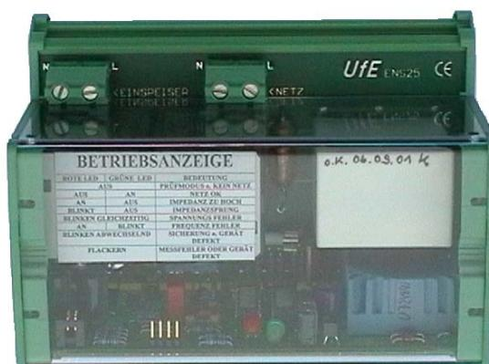
The ENS25 is an autonomous release unit according to DIN VDE0126. This way the unit replaces the always accessible release mechanism of the power supplier.
